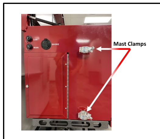
Figure 5. Command Runner Mast Mount Location
